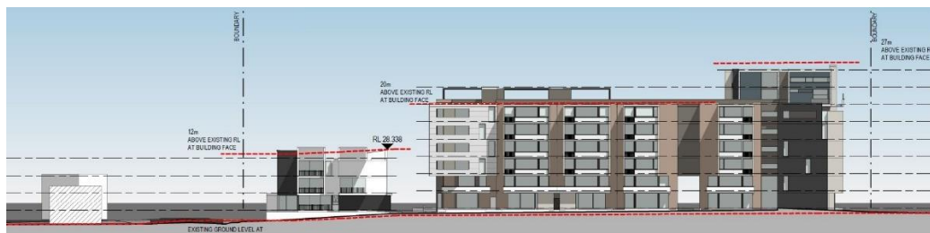
Figure 31 - Southern elevation of building C3, C2 and C1 showing the transition in scale from Queen Street to the rear portion of the site further east (Source: AJ + C, Drawing No DA3100, Rev B, 17.08.17)
